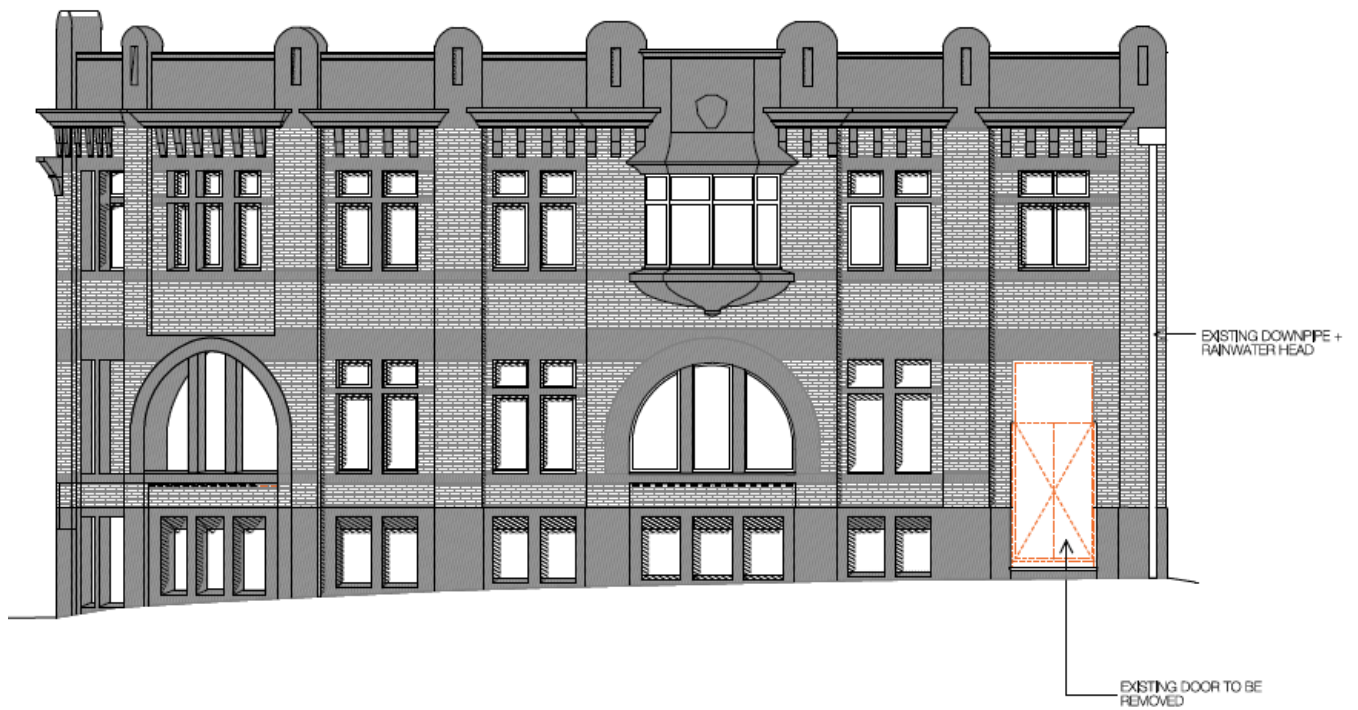
Figure 26: Bourke Street (west) elevation demolition plan
