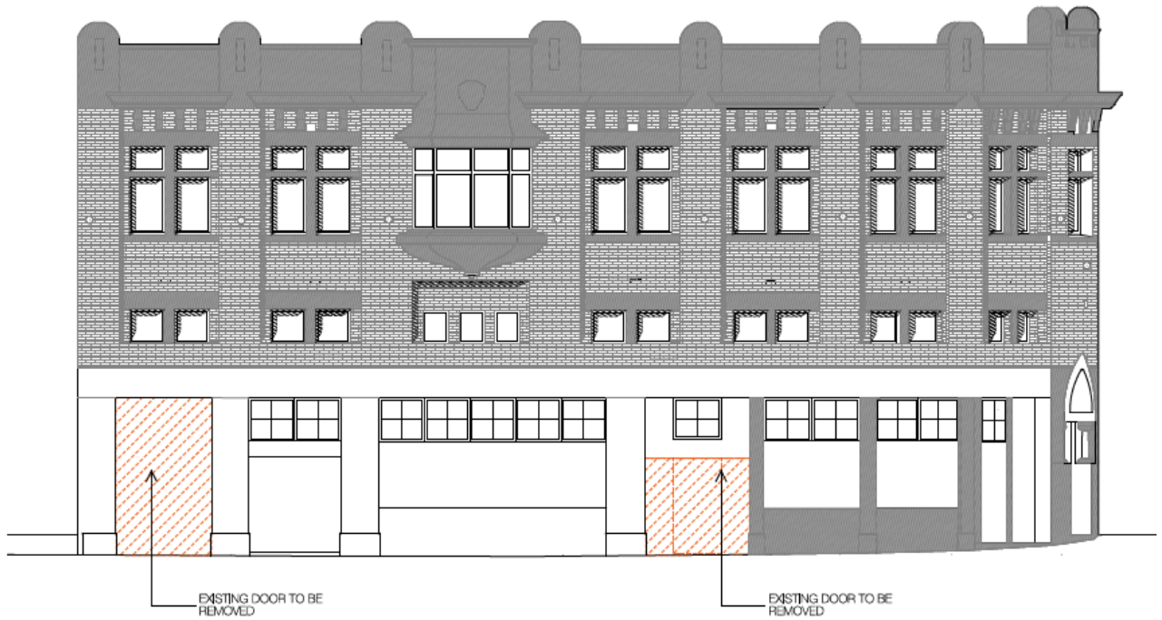
Figure 27: Flinders Street (east) elevation demolition plan
