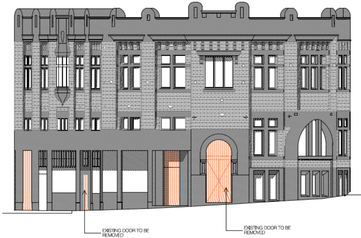
Figure 25: Taylor Square (north) elevation demolition plan
