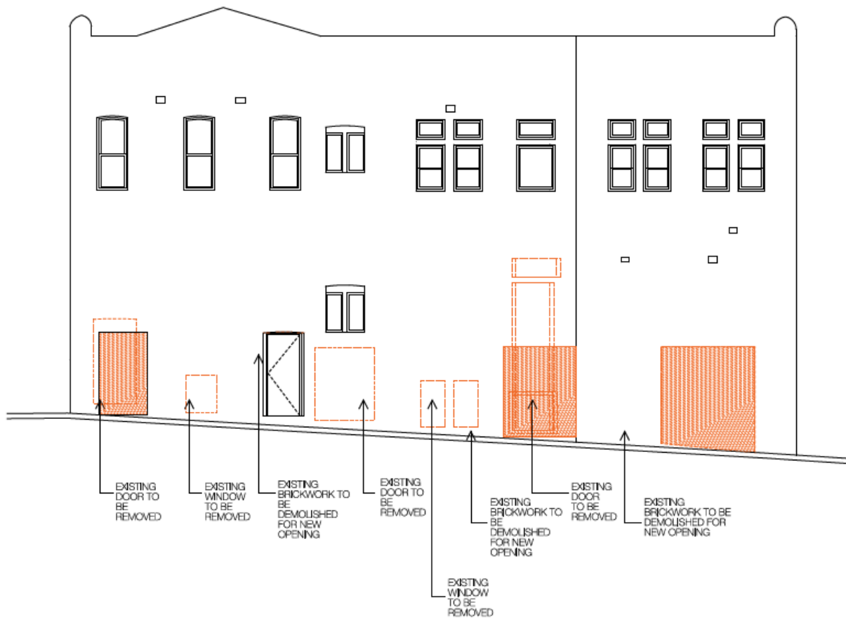
Figure 28: Patterson Lane (south) elevation demolition plan
